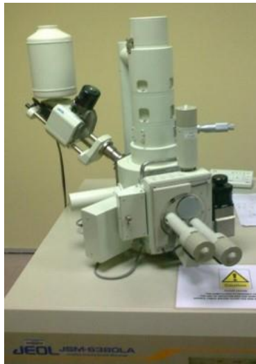
Figure 3-2: SEM machine with EDS (Model: JSM 6380 La)
