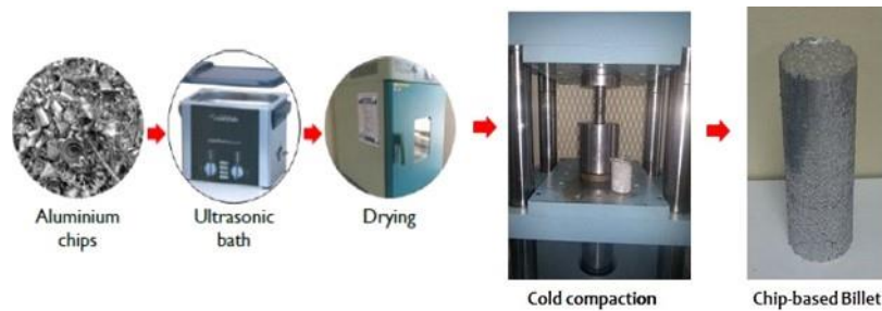
Figure 3-3: Pre-processing of chips before extrusion
