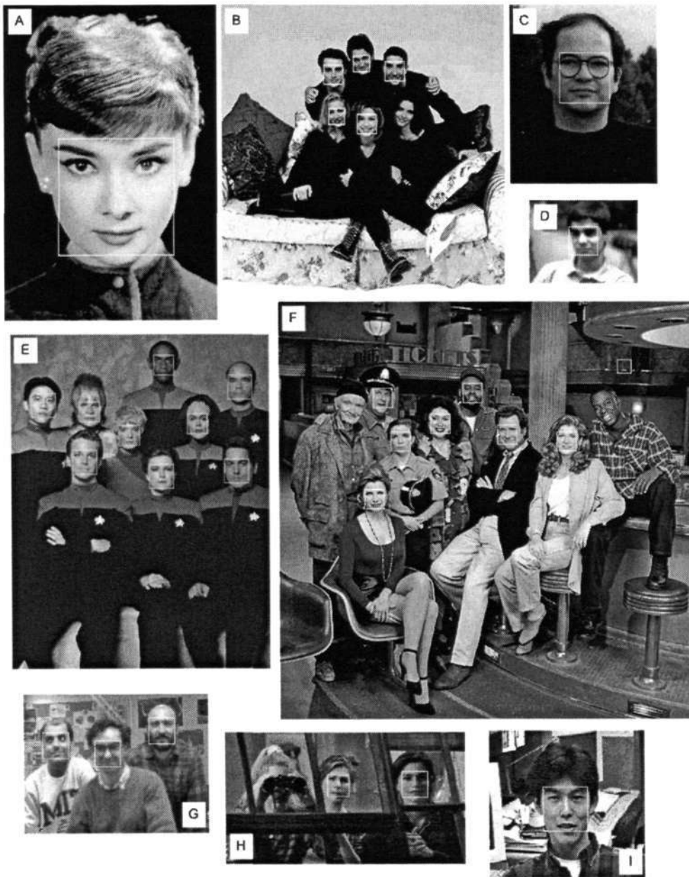
Figure 3.4: Some results on test images. The detected faces are framed in white. There are missed detections in (B,F,H), and a false detection in (F). The missed detections are due to severe rotation or large occlusion. The face detection is on a subregion which is quite like a real face.
