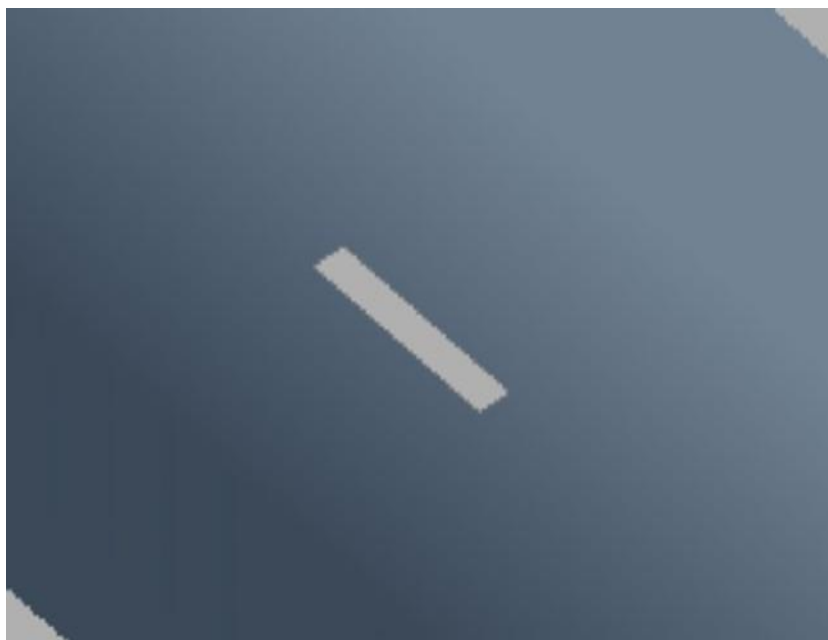
Figure 7.2 The chip for in situ TEM with a window in the center.
