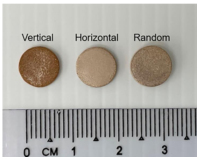
Figure S3. The color difference of BN-PVP composites with different oriented microstructures prepared by MASC.
