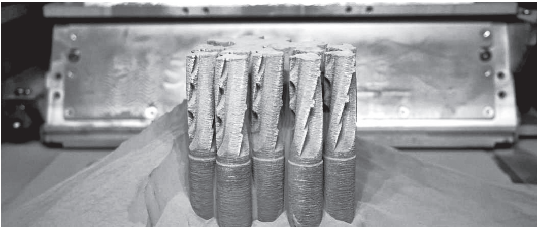
Figure 5. Additively manufactured cutter shafts
