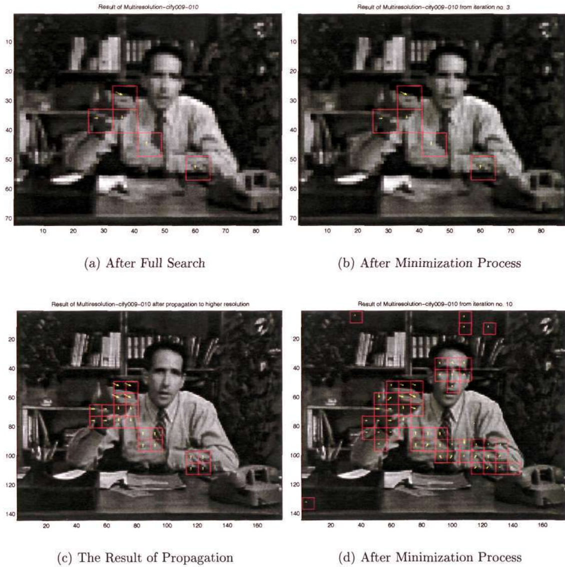
Figure 5.31: Results of Multiresolution Block Matching with Smoothness Prior for the Salesman Sequence.
