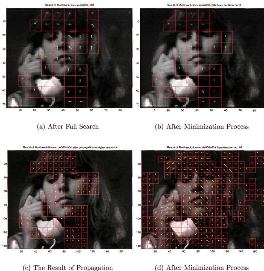
Figure 5.25: Results of Multiresolution Block Matching with Smoothness Prior for the Suzie Sequence.
