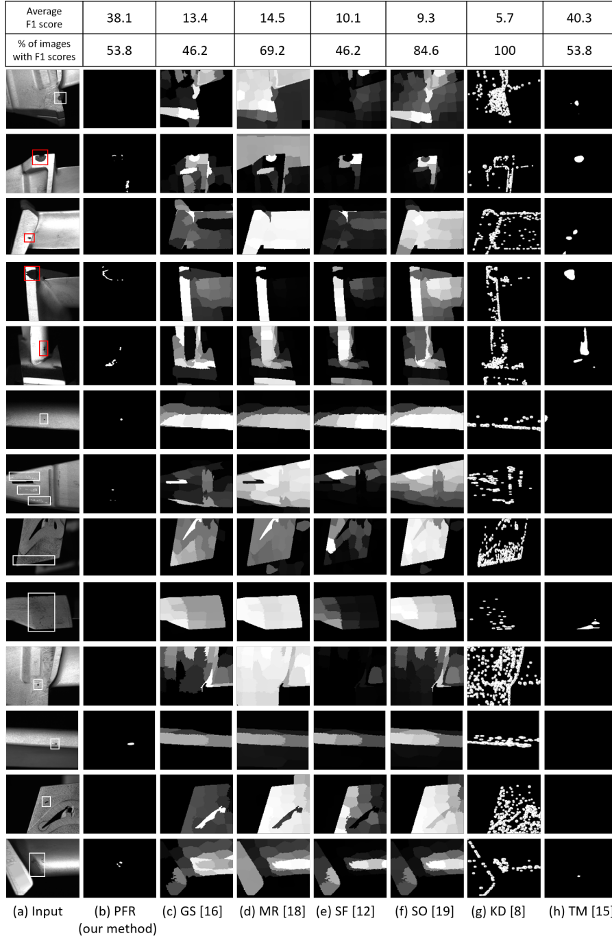
Fig. 6: Saliency maps from different anomaly detection methods applying on bright images. (a) Bright images with bounding boxes indicating locations of anomalies, (b) results from the proposed PFR, (c) Geodesic Saliency (GS) [16], (d) Manifold Ranking (MR) [18], (e) Saliency Filter (SF) [12], (f) Saliency Optimization (SO) [19], (g) Keypoint Detection (KD) [8], and (h) Template Matching (TM) [15].
