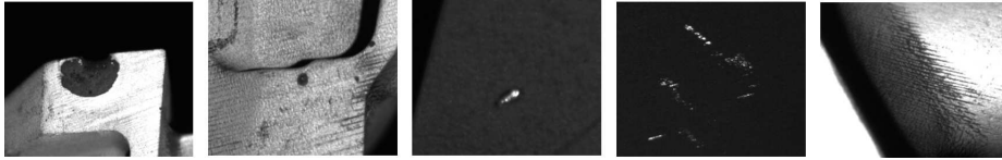
Fig. 2: Example of anomalies. From left to right are melt, plus metal, scratch, scuff and shadowing.
