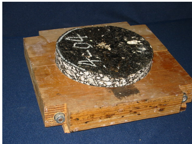
Figure 4.14 WWT Set Up for the Wheel Tracking Test
