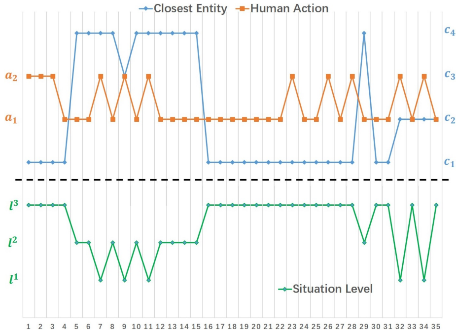
Figure 14: The inferred result of the level of the situation in Dataset 3. The figure above shows the target action and the closest entity to the target at each decision step. The figure below shows inferred levels of the current situation. It indicates that the situation level is easy at decision steps 7, 9, 11, 32, 34.
