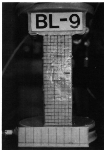
Fig. 2.20 Typical deformation mode of a loose specimen at the end of plane-strain test (after Han & Vardoulakis, 1991)
