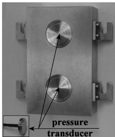
Fig. 3.4 The lateral loading platen
