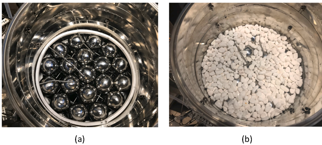
Fig. 17. A packed-bed CTES with two types of fillers: (a) macroencapsulated PCM; and b) granular (quartzite pebbles) inserted in the gaps between the sphere tiers [180].
