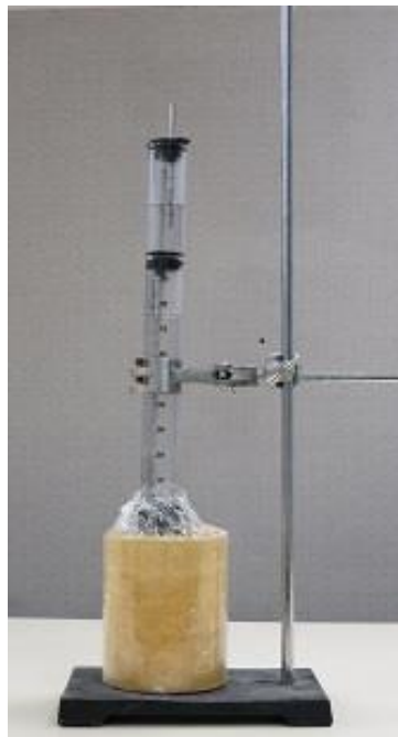
Figure 3.11: Infiltration test using a mini-disk infiltrometer
