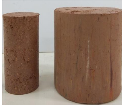
Figure 3.6: Typical compaction specimens, left specimen obtained using the PVC mould and the right specimen using the ASTM standard compaction mould
