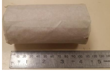
Figure 3.13: Compacted sample prepared for sawing to obtain BTS test specimens
