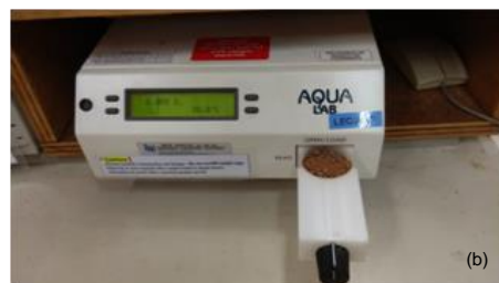
Figure 3.9: Mounting a test specimen with the chilled mirror hygrometer
