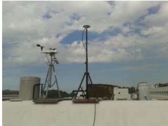
Figure 3-3 Septentrio GNSS antenna
