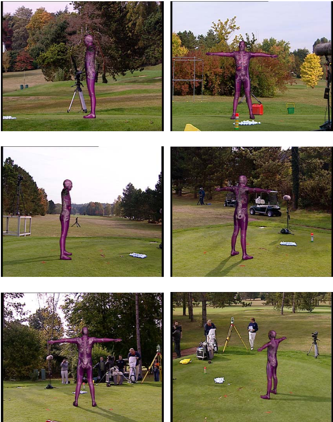
Figure 6.7. 3D Model of the 'big-man' superimposed onto the images from 6 different views (model refinement using silhouette)
