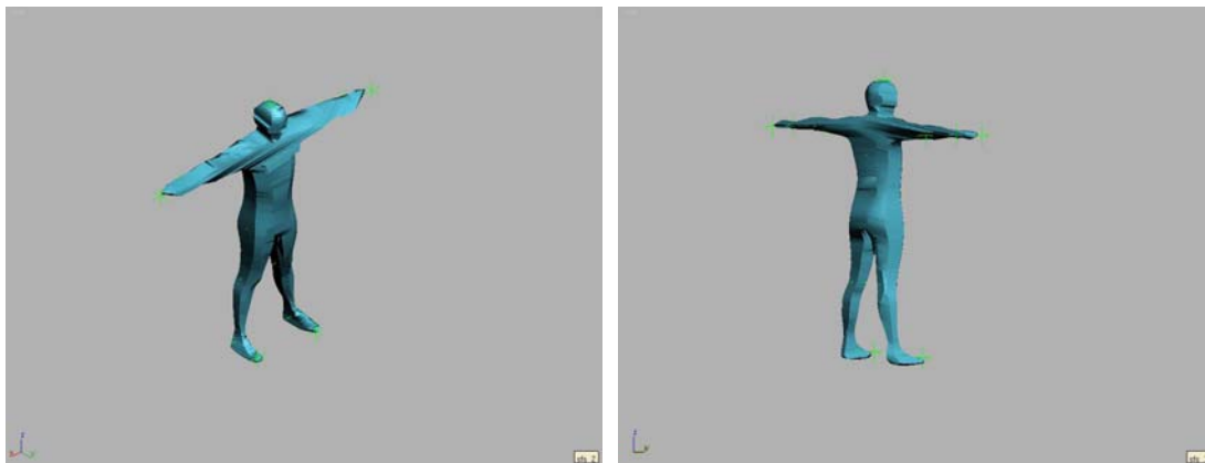
Figure 2.3. Shape-from-silhouette using 6 cameras. Some parts of the body are very blocky and unreal.
