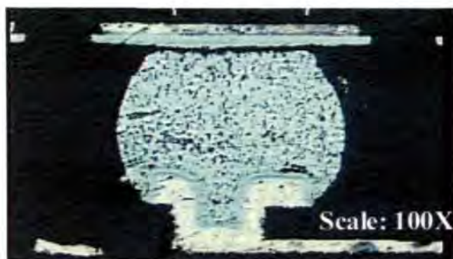
Figure 5.4. Failure analysis of solder ball
