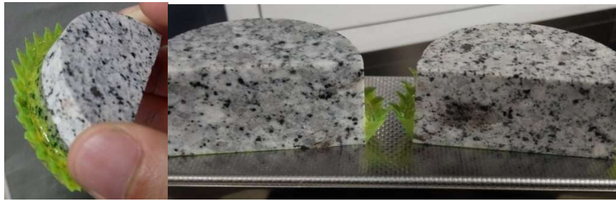
Fig. 3.6 Specimens coated with fluorescent epoxy (50 mm diameter)
