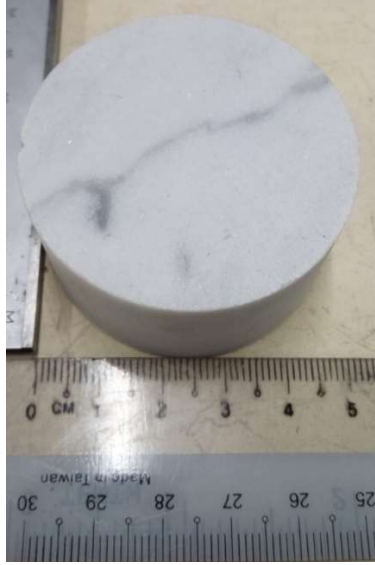
Fig. 3.4 Carrara marble specimen (around 48 mm in diameter, around 26 mm in thickness)
