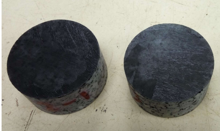
Fig. 3.14 Granite specimens (50 mm diameter, thickness of around 25 mm) coated with high temperature grease to simulate soot and smoke damage.
