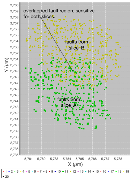
Fig. 10: Slice-exclusive faults for a single CLB.
