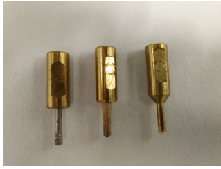
Fig. 2: ASAP-1 tools. From left to right: Diamond tool, Xylem tool and Xybove tool.
