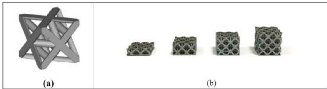
Fig. 12 (a) Unit of Octet-truss and (b) porous structures of height range 2.5 mm to 10 mm fabricated by Wong et al. [107].
