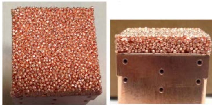
Fig. 7 Photographs of surface produced by particle sintering with particle size of 850-1000 \mu\text{m} (a) top view (b) side view [73].
