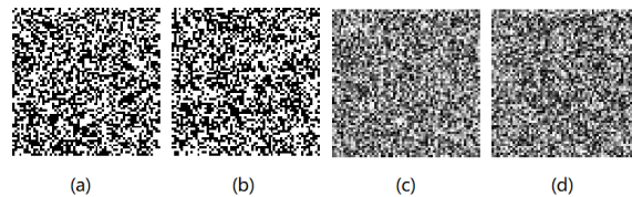
Fig. 4. (a)-(b) 2D patterns derived from the initial Hadamard matrix and (c)-(d) the corresponding phase only profiles retrieved from (a) and (b).
