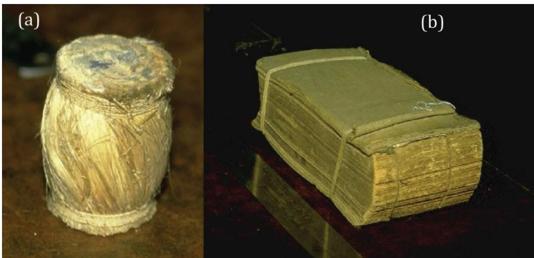
Figure 1.2: Artificial material medium demonstrate by J. C Bose. a) Twisted-jute polarizer for polarization rotation, b) Linear polarizer consisting of a book pages interleaved with tinfoils.
