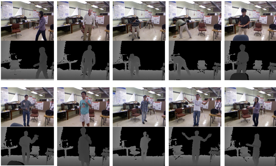
Fig. 2.13 Illustration of the RGB frames and corresponding depth-maps from different samples in UTKinect dataset.
