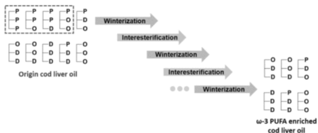
Fig. 1 Illustration of the proposed method to enrich omega-3 PUFA in CLO in TAG form via alternate operation of solvent winterization and enzymatic interesterification. (P, palmitic; O, oleic; D, DHA. The designation POD, etc., does not imply the TAG POD alone, but a mixture of all positional isomers — POD, ODP and PDO, etc.).
