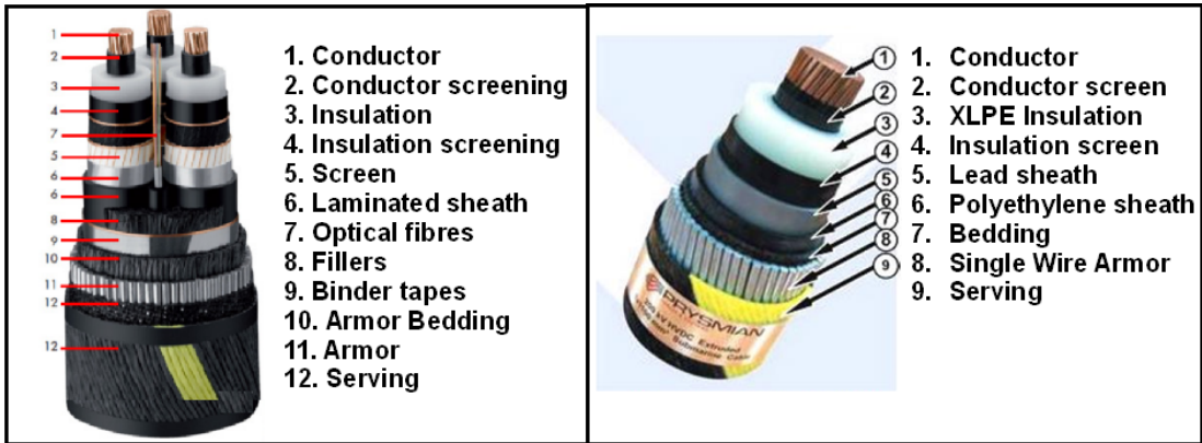
Figure 2.3: Typical cable components of (i) HVAC [5] subsea cables and (ii) HVDC subsea Cables [6]
