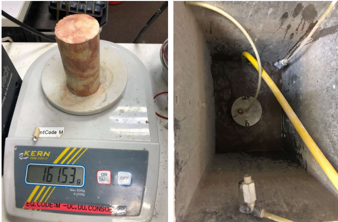
Figure A.3: Test set-up for falling-head permeability test
