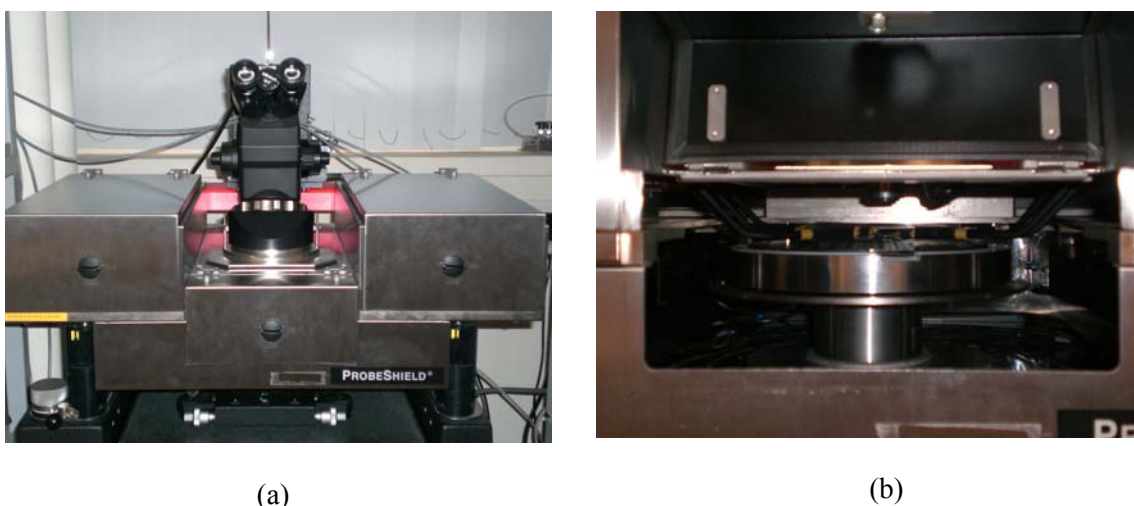
Fig. 3.2 (a) Front view of the Suss MicroTec probe station used in this project with closed prober shield. (b) The test wafer is carefully placed on the thermal chuck of the probe station with tight suction provided by the vacuum pump.
