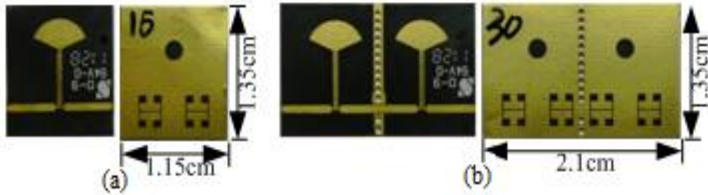
Figure 3.7 (a) Top view and bottom views of one-cell TRS LPF; (b) Top and bottom views of two-cell TRS LPF.
