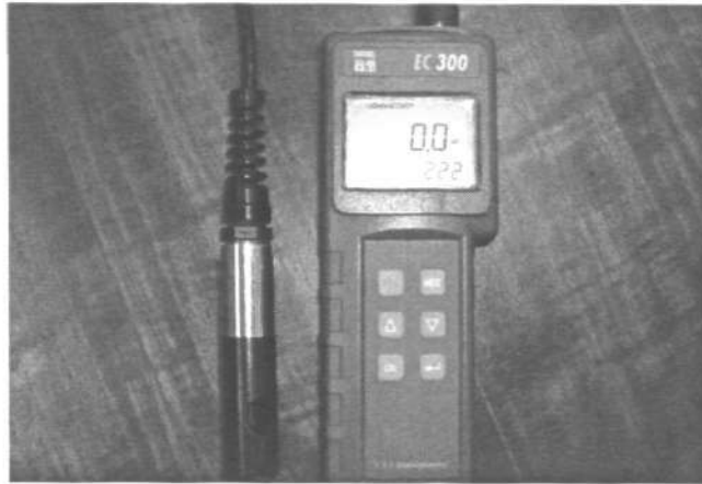
Figure 4.8 - The commercial conductivity meter (YSI model EC300).
