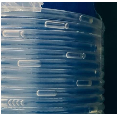
Figure 6.2 Photograph of the gas bubble trains and the liquid slugs containing the crystallization solution from the base case SFC design
