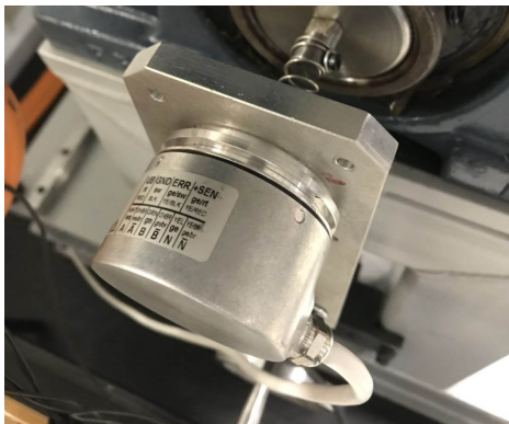
(a) Installed Encoder
