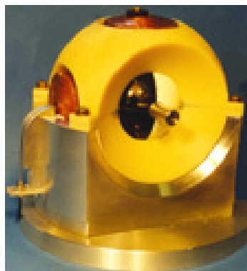
Figure 1.19. Wang et al. spherical permanent magnet motor.
