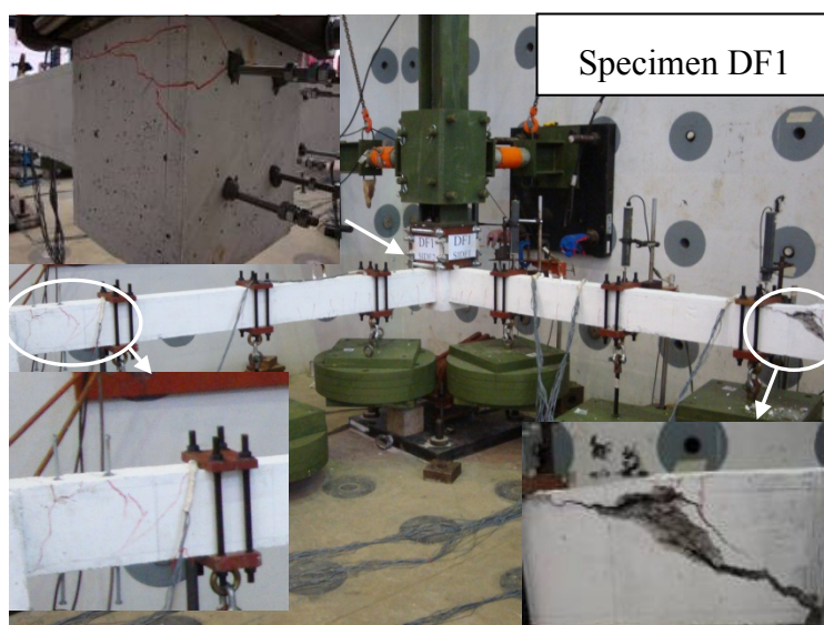
Fig. 6.5: Observed crack pattern of DF1 after test
