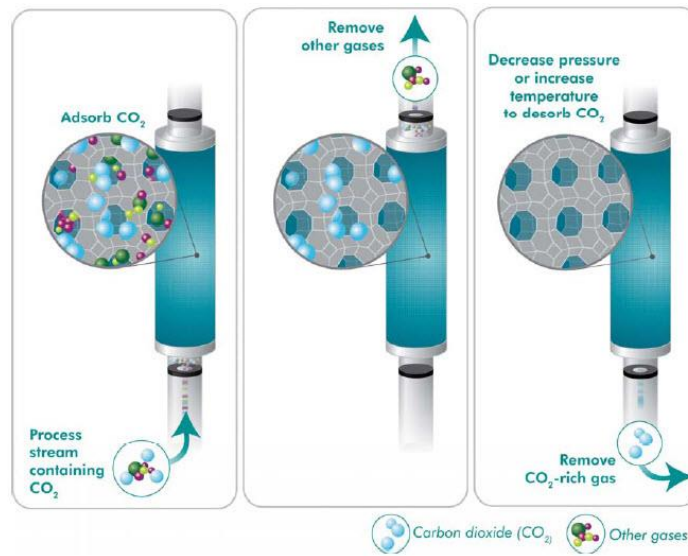
Figure 1-2 Illustration diagrams of physical adsorption process for carbon dioxide separation[8].
