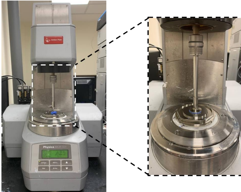
Figure 3.1 Anton Paar MCR 501 rotational rheometer which was used in this thesis with a parallel plate spindle.
