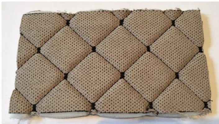
Figure 7.8 Soft composite concept where PBS is the middle layer closed by 3D fabric from two sides and stitched over the area.
