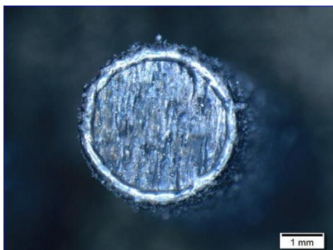
Figure 4. Microscopic views of (a) circular, (b) rectangular rounded and (c) aerofoil fins.
