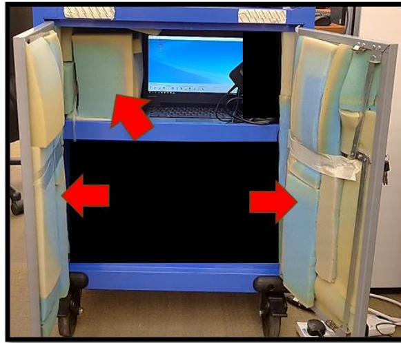
Figure 3-3. The IAQ station, inside the station where the sampling pumps were kept and locked. The doors were cushioned with thick sponges to absorb the noise from the equipment. The noisy sampling pump had an additional cushioning layer to create an enclosed environment to reduce noise.
