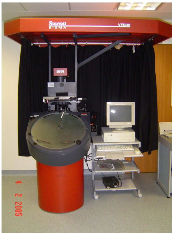
Figure 3.3: A photograph of Starrett Sigma vertical optical profile projector (VF600).
