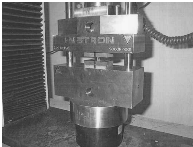
Figure 3.5: A photograph of Illinois Institute of Technology Research Institute (IITRI) compression test-rig.
