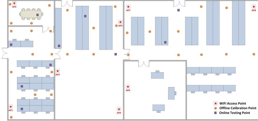
Figure 5.2: Positions of the WiFi access points, offline calibration points and online testing points in the test-bed
