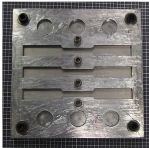
Figure A4 Image of dog-bone/round disk shaped mold.
