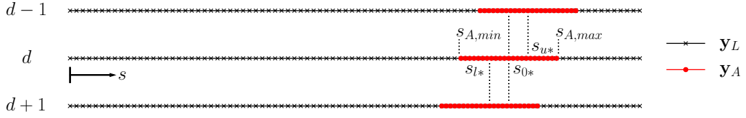
Figure 4.4: Prepared line discretisations with staggered refined segments.
