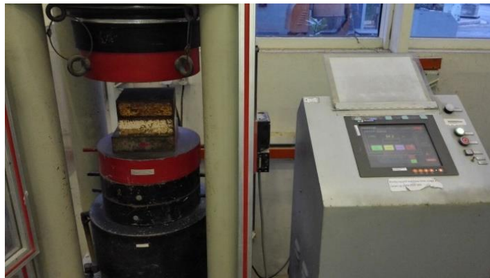
Fig. 5.3. Set-up for compressive test.
