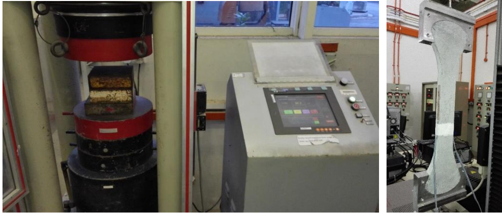
Fig. 3.1. Test setup (a). compressive and splitting tensile testing machine (b). uniaxial tensile testing machine.
