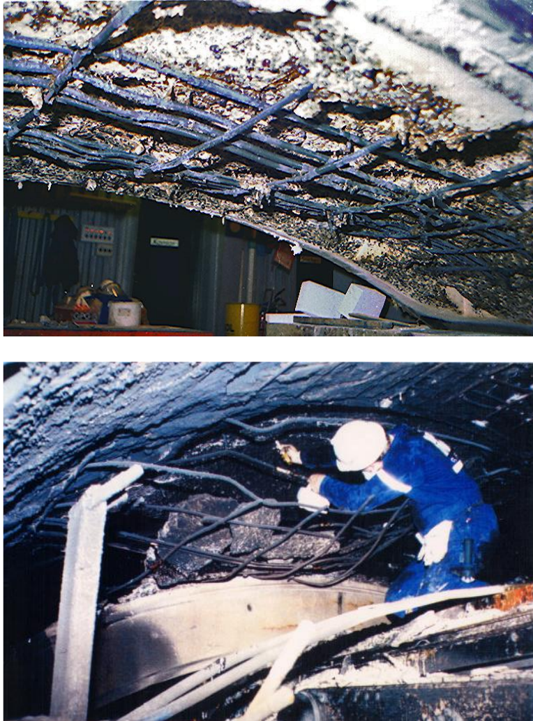
Fig. 1.1. Tunnel element from the Great Belt tunnel fire tested at SP Technical Research Institute of Sweden (Jansson 2013, Khoury and Anderberg 2000).
