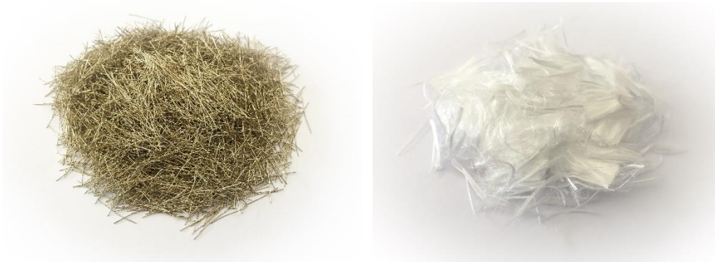
Fig. 5.1. Micro steel fibers and PE fibers used in this study.
