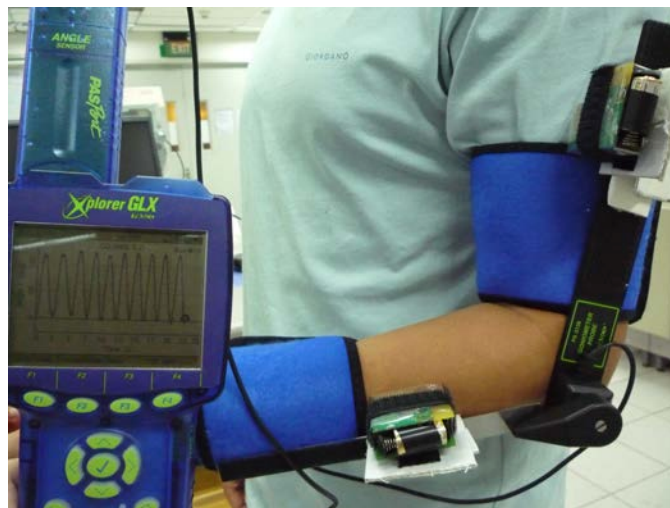
Figure 4.9. Attachment of the sensor nodes and goniometer to a human arm
