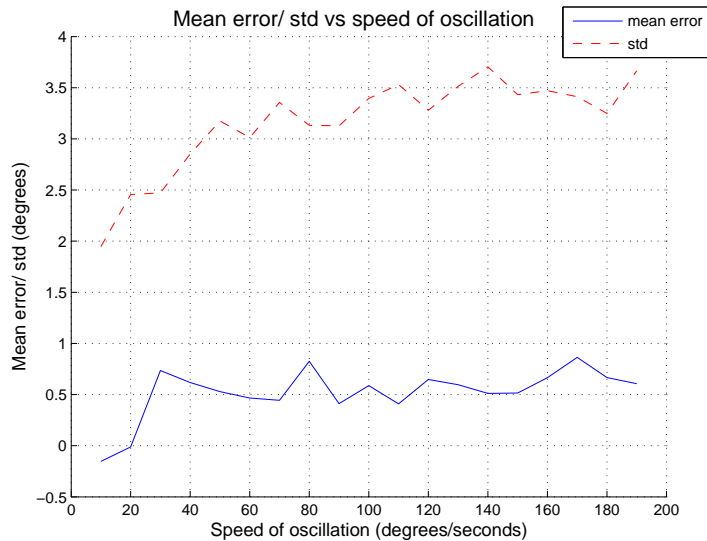
Figure 4.7. Mean error and variance of accelerometer readings at different speeds of oscillation
