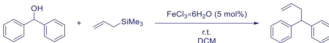
Scheme 2.5. Iron chloride catalyzed deoxygenative allylation
