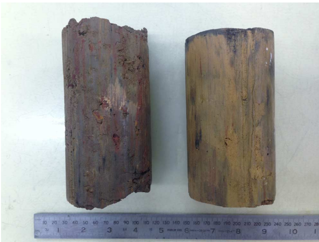
FIG. 6 Residual soil specimens from Jurong Formation, Singapore. Left: clayey sand; Right: clay.
