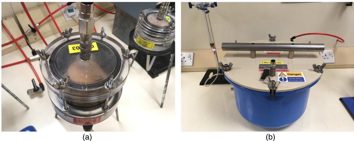
FIG. 4 Pressure chambers using the axis-translation method. (a) Tempe cell; (b) pressure plate.
