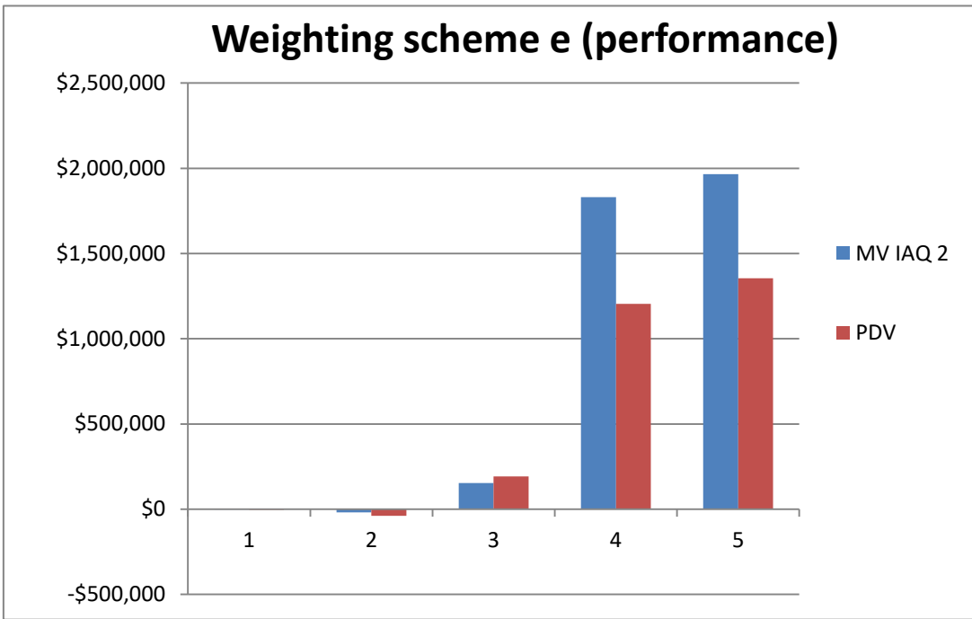
Figure 4.7 Weighting scheme e (performance): 1: Extra ACMV capital expenses; 2: Extra operational energy expenses; 3: Benefits of avoided sick leave; 4: Benefits of increased average mark; 5: Total net benefits. The Benefits to Extra Expenses Ratios: (a) MV IAQ 2: 104.2; (b) PDV: 33.1. All values are relative to the MV IAQ 1 scenario.
