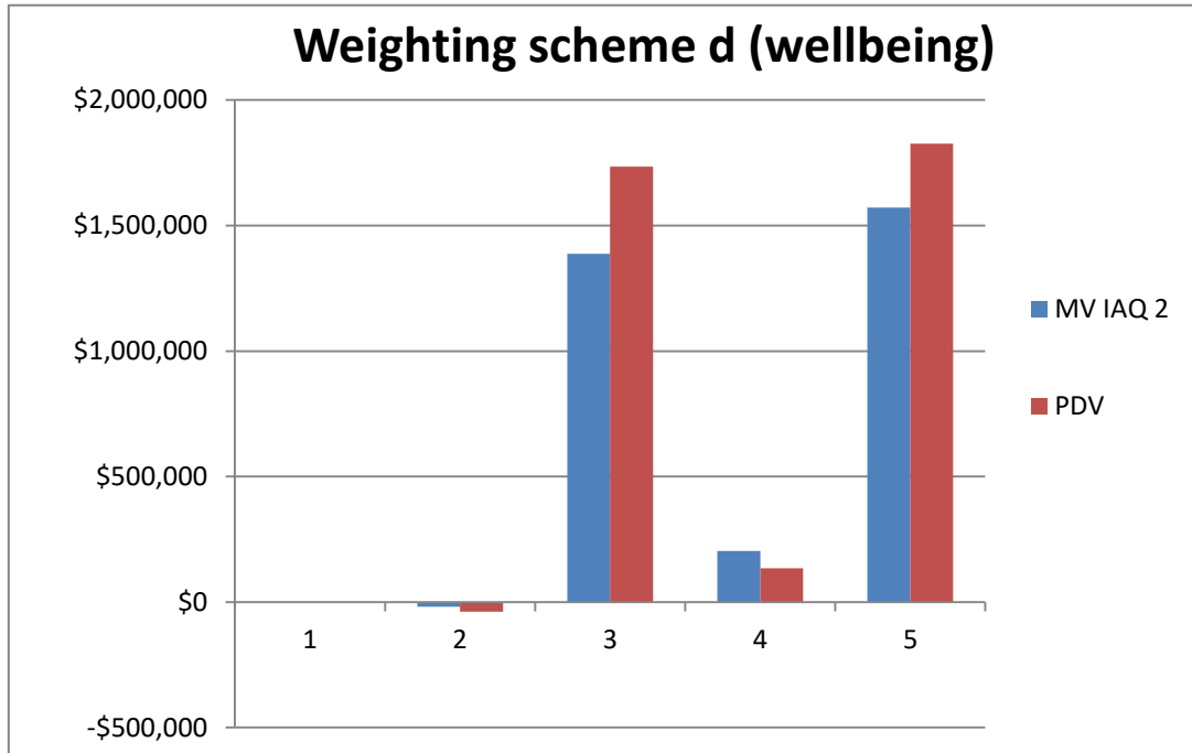
Figure 4.6 Weighting scheme d (wellbeing): 1: Extra ACMV capital expenses; 2: Extra operational energy expenses; 3: Benefits of avoided sick leave; 4: Benefits of increased average mark; 5: Total net benefits. The Benefits to Extra Expenses Ratios: (a) MV IAQ 2: 83.5; (b) PDV: 44.2. All values are relative to the MV IAQ 1 scenario.
