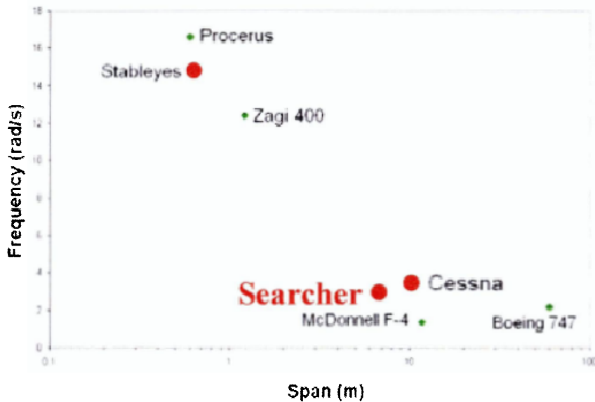
Figure 5.8: Short Period natural frequency plotted versus span for various aircrafts
