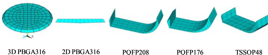
Fig. 4-10 Averaged volumes located on component side for different assemblies.
