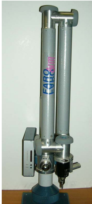
Figure 24 High definition digitizer (FaroArm) with ball probe used to capture geometrical details of vertebrae.
