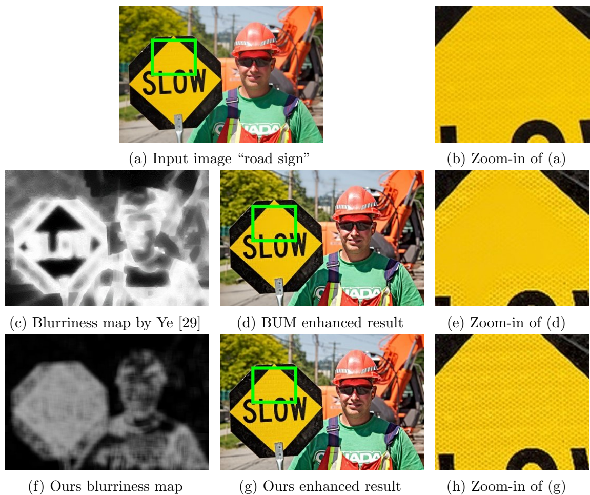
FIGURE 4.9: Comparison of the blurriness estimation and BUM result with the “road sign” image.
