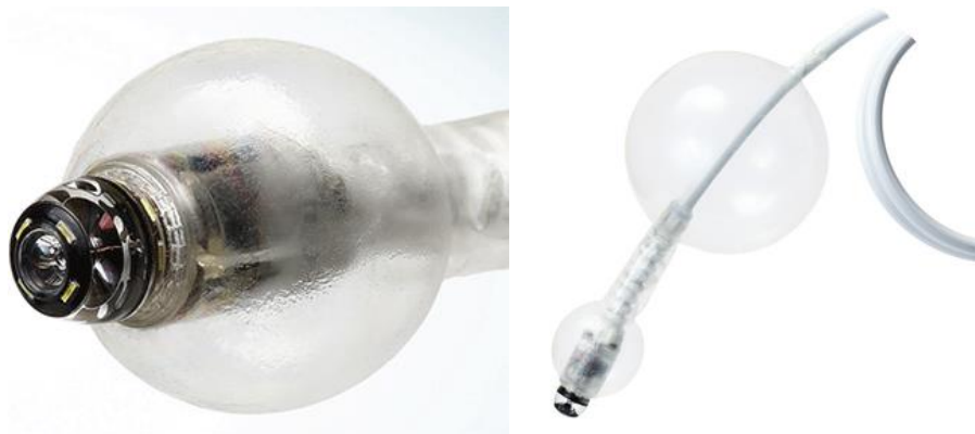
Fig. 1: Omni-view cameras on tip of endoscope with inflated distal balloon. Reproduced with permission. Source [ http://www.giview.com/contact-us.html ]
