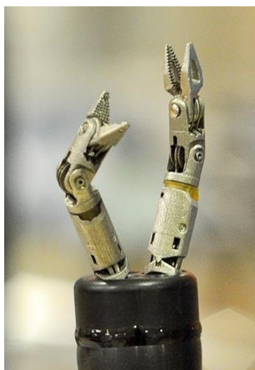
Fig. 9: Twin 7 DOF arms on Endomaster's MASTER robot. Reproduced with permission. Source: [www.endomastermedical.com]
