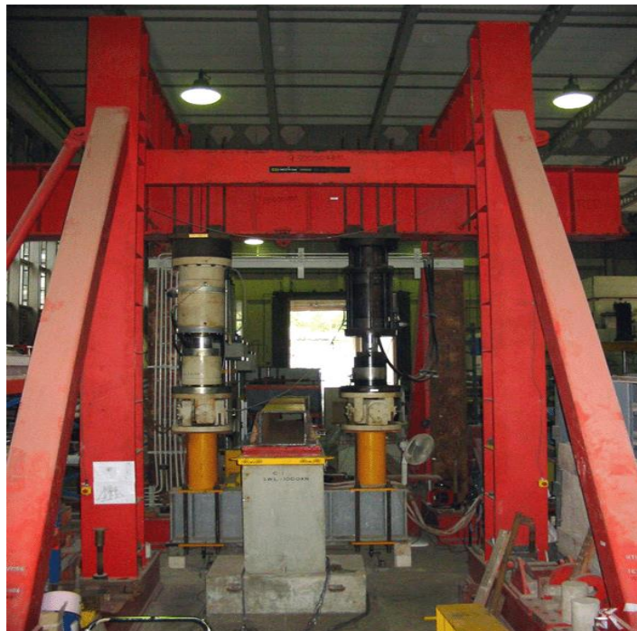
Fig. 7 Test rig for SHS T-joint [11]
