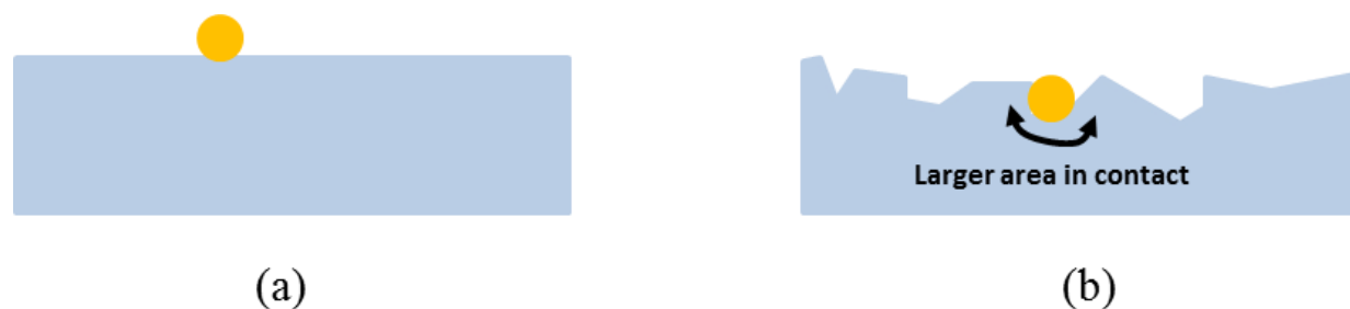
Figure 5-12: Schematic illustration of area in contact of an atom on a (a) smooth surface and (b) rough surface
